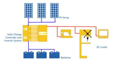
Figure 2.3: Layout of a PV - battery off-grid system **Source:** adopted from Alsharif, Nordin and Ismail, (2015)
