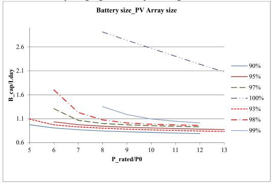
Figure 3.1: System combination curves PV array size and the corresponding battery size
