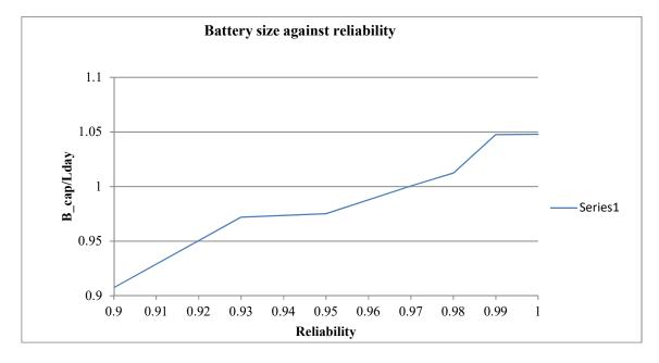
Figure 3.5: Normalised battery capacity against Reliability
