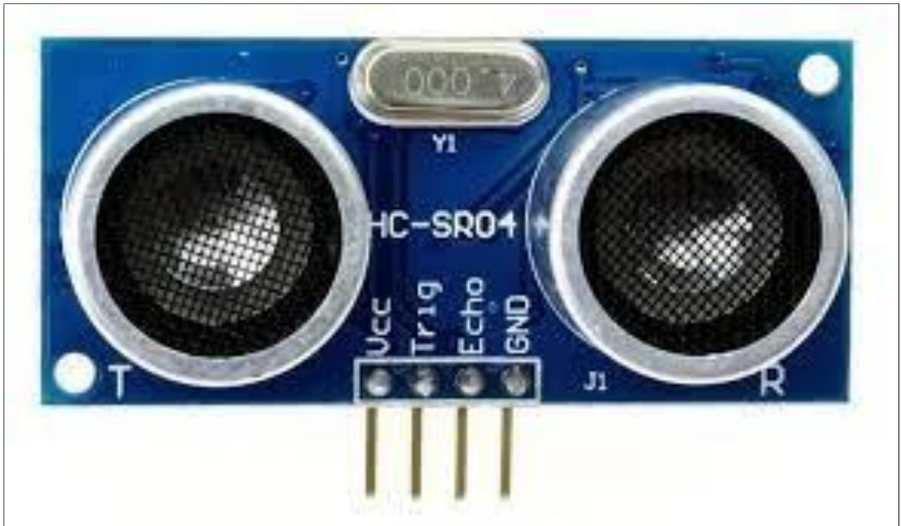
Figure 1: Ultrasonic sensor
