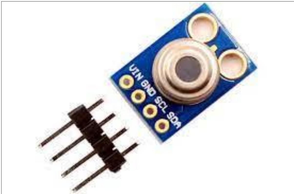
Figure 2: MLX90614 wireless temperature sensor
